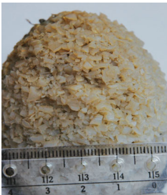
Figure 2 Granulated PTFE particles (in cm). [Color figure can be viewed in the online issue, which is available at www.interscience.wiley.com .]
